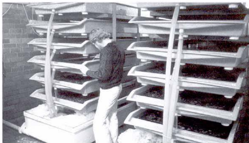
An oyster purification plant in New South Wales. Clean water is continually circulated through the racks.
