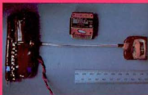
The electronic activity recorder (EAR), designed and built by Mr Kit Williams. The larger part fits on the penguin's back, and consists of the depth transducer, batteries, and memory. The small unit, worn on the front of the bird, contains the speed transducer. They are connected by the attachment ribbon that wraps around the penguin.
