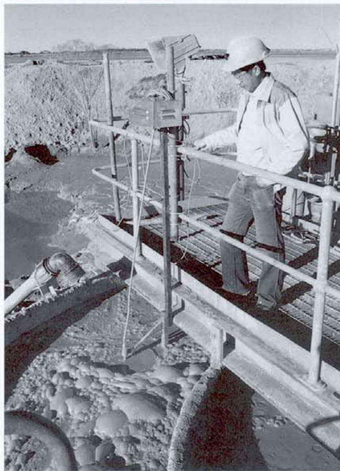
When activated carbon is added to the powdered gold and cyanide solution, it selectively adsorbs the gold. Here, Dr Paul Fung tests a sample of his jarrah carbon pellets.
