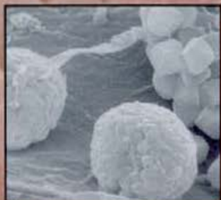
Pyrite occurs in a number of forms (big picture and above): crystalline granules, spheres and flattened sheets that are actually 'fossilised' leaves formed by pyrite molecules replacing organic substances.
