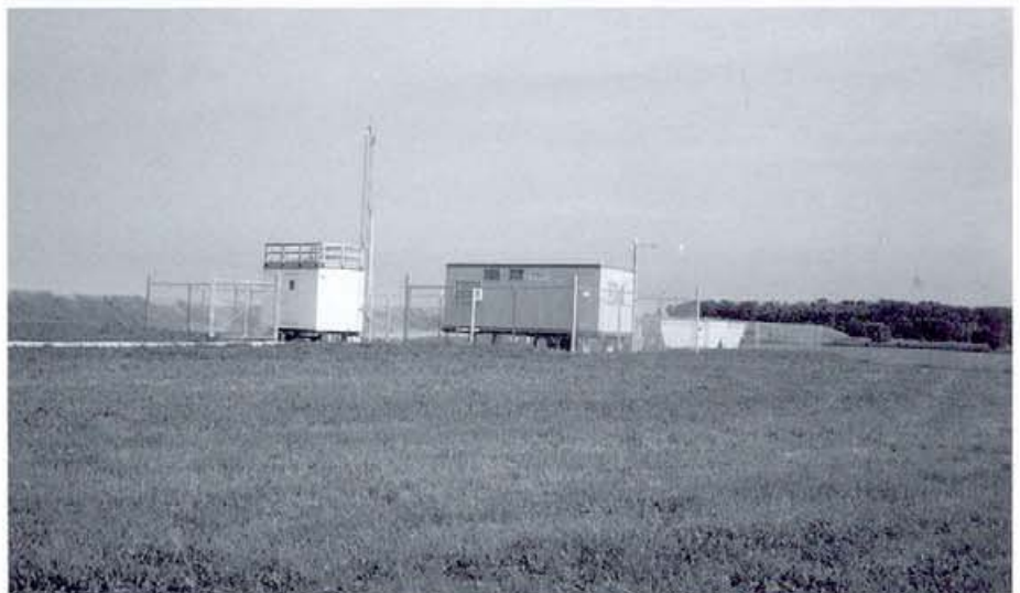
One of four Airtrak monitoring stations used in a photochemical smog study in the Chicago/Lake Michigan area of the United States.
