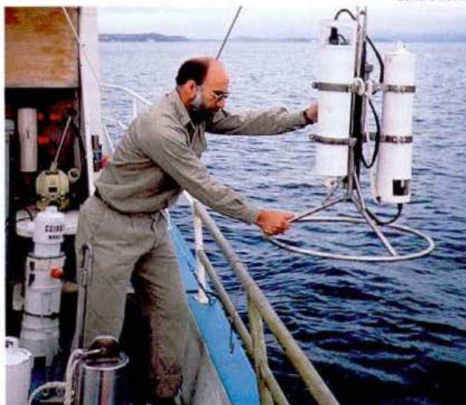
Deploying instruments for trace metal measurement in Macquarie Harbour.
