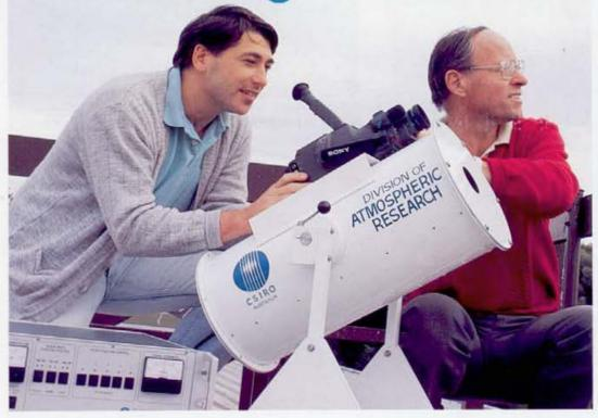
Dr Fred Prata (left) and Dr Ian Barton with a prototype of the AVADS volcanic ash detector. The instrument can be mounted on an aircraft wing or in the nose.
