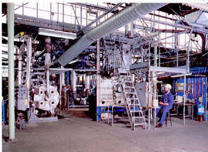
At the Division of Coal and Energy Technology, North Ryde laboratories, a miniature pulverised-coal-fired boiler is helping researchers improve the performance of power stations.
