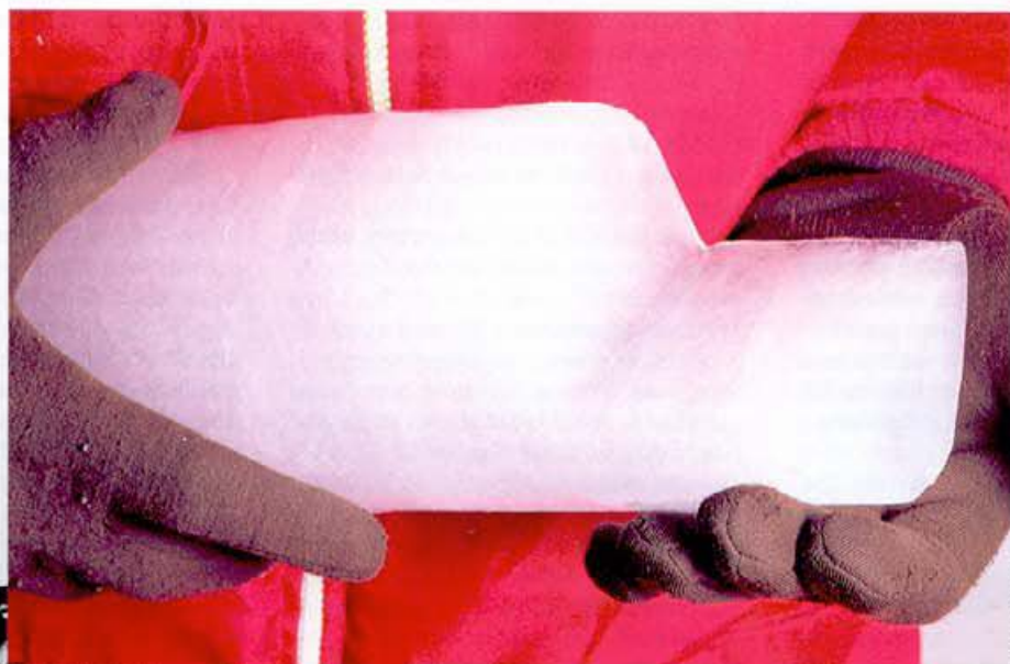
An ice sample, from a depth of about 300m, cut off for gas analysis.
