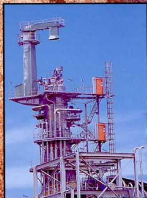
Main picture: Woodchips ready for pulping at the APM mill in Gippsland, Victoria. Inset above (left to right): Unbleached, partially bleached and bleached eucalypt kraft pulp. Right: Pulping takes place in the continuous digester.
