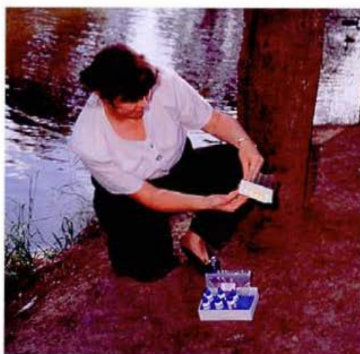
Low cost, sensitivity and speed are the key features of the compact Elisa kit, which tracks pesticides and herbicides in the environment.
