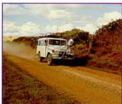
Lower right: Cross-wind plume measurements were taken from a four-wheel-drive vehicle travelling at right angles to the plume direction. The concentrations of emissions such as sulfur dioxide and nitrogen oxides were recorded.
