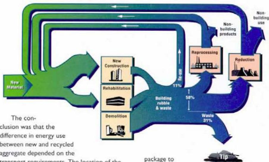
The conclusion was that the difference in energy use between new and recycled aggregate depended on the transport requirements. The location of the crushing plant in relation to the supply of salvaged concrete is important. If old concrete has to be returned to a distant quarry for crushing, the energy cost is high. Tucker says the exercise has demonstrated a useful principle for ascertaining embodied energy in construction materials and techniques.
