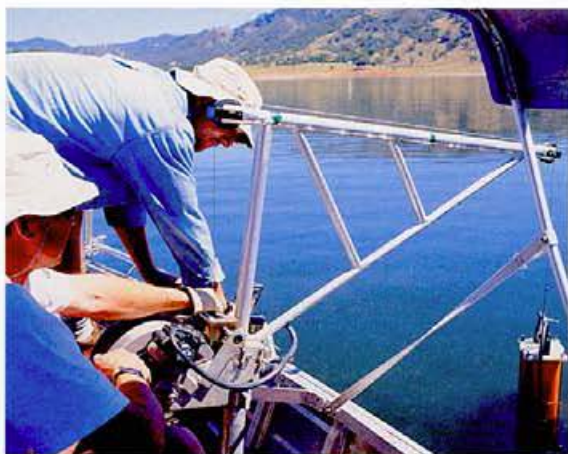
Above: Patrick Hatton and Bruce Hindmarsh prepare to measure a profile of temperature, dissolved oxygen and chlorophyll fluorescence at Chaffey Dam. Left: A bubble plume hits the surface.
