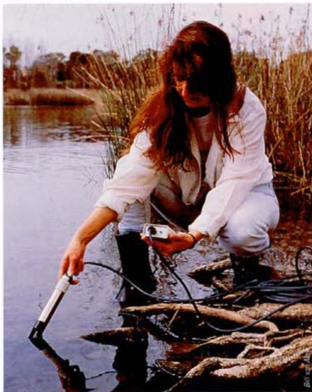
Measuring the rate at which microbes consume oxygen has been simplified with the development by CSIRO and Greenspan of a durable and reliable dissolved oxygen probe. Yvette Oliver from CSIRO's Division of Water Resources demonstrates the instrument which uses a diffusion cell to measure oxygen in gas, surface water and groundwater.
