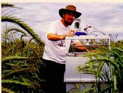
Dr Mick Meyer from the Division of Atmospheric Research calibrates an automated gas exchange chamber in a triticale crop during the OASIS experiment at Wagga.
