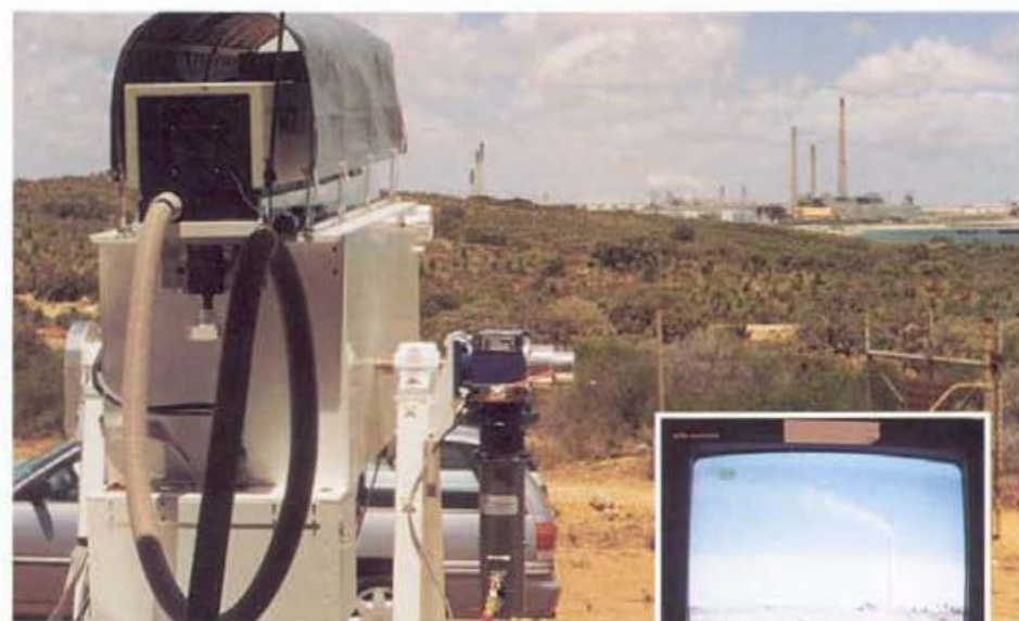
Above: Tracking the plume from Kwinana's power station as it mixes with the atmosphere. The lidar measurements helped to validate a plume-dispersion model used to determine ground-level concentrations of sulfur dioxide.
