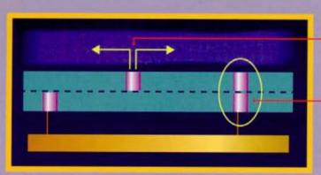
The biosensor can detect the presence of specific particles, and signal their presence by triggering an electrical current. It combines two, nanoscale building blocks: a sliding switch and an electrode.
