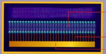
The electrode has a miniature reservoir formed between its surface and a biological membrane made from two layers of lipids. The 'bottom' layer of lipid is attached to the electrode by linking molecules. A slice through the membrane is illustrated below. The 'outer' half channels can move around in the top layer of the membrane
