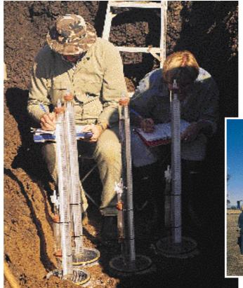
Left: Hydrologic measurements were taken to help determine how quickly water flows beyond crop roots. Below: Drilling holes for the installation of groundwater monitoring equipment.
