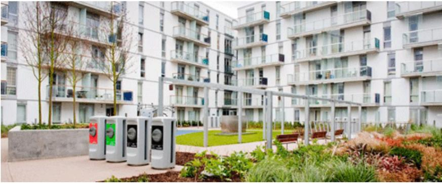
Vacuum waste inlets, Wembley City, UK. Vacuum waste systems use suction pipes to transfer waste to a central treatment plant. The scale of Wembley City facilitates use of technologies such as this that may not be feasible on a smaller scale.
